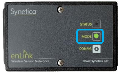
Blinking Green LED – Device Successfully Joined
